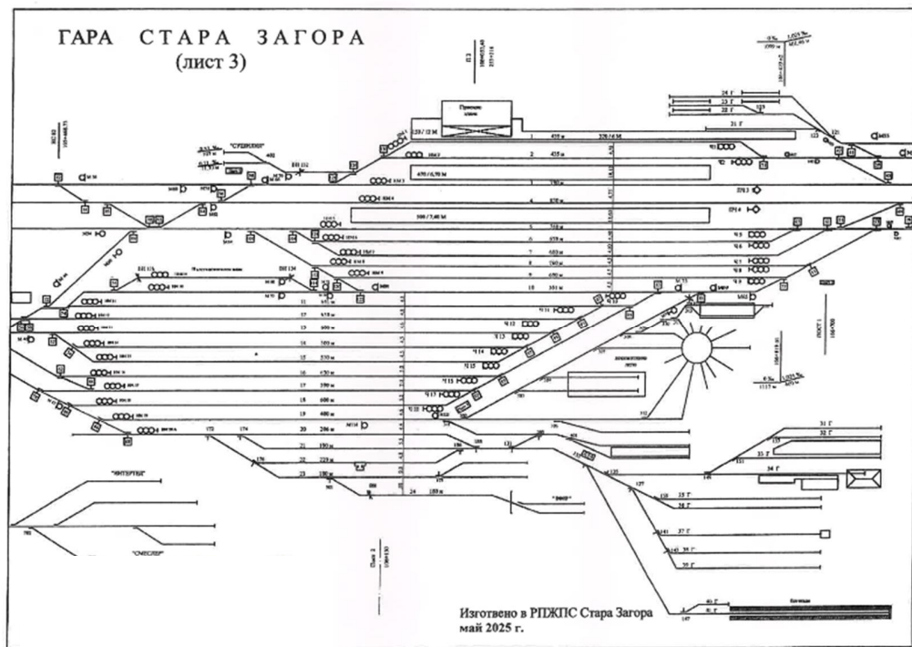
Fig. 3.4. Scheme of Stara Zagora station
