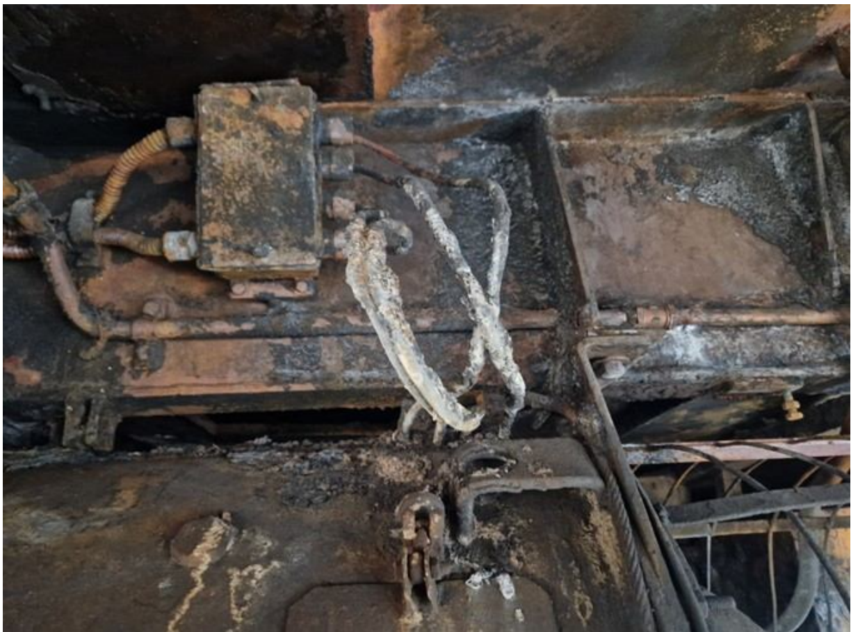
Fig. 4.18. Power supplying cables of first under body shell engine fan
