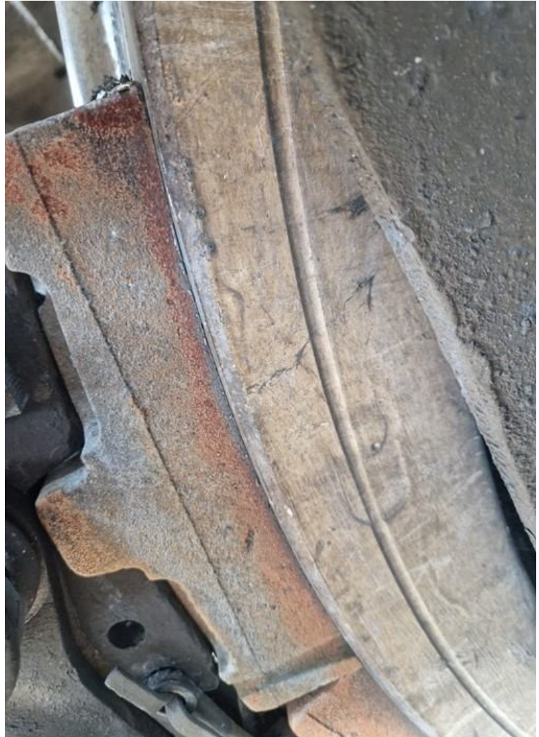
Fig. 4.19. Condition of the locomotive pad
