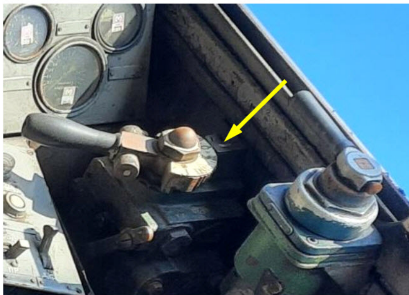
Fig. 4.32, pos. 2. The switch shows that the brake valve for the automatic brake is on an insulated position .
