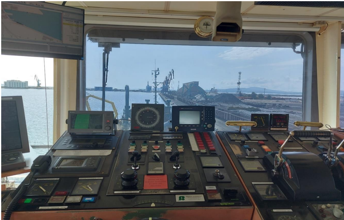
Fig. 1 – Navigation control panel on the bridge of the dredger "MILFORD"
