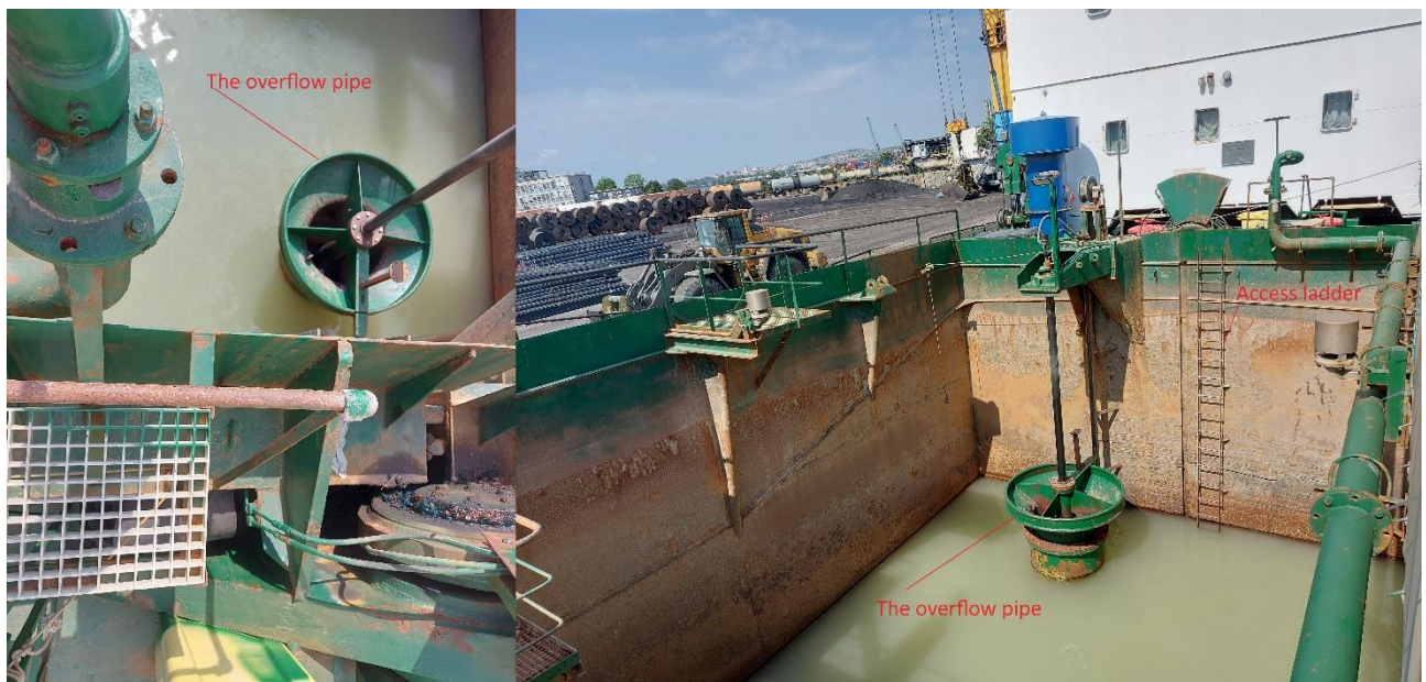
Fig . 4 – Overflow device and gangway for access to the cargo tank of dredger "MILFORD".
